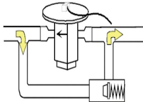
Most expansion valves used in current Goodman/Amana® Brand Heat Pump products use an internally checked expansion valve.
