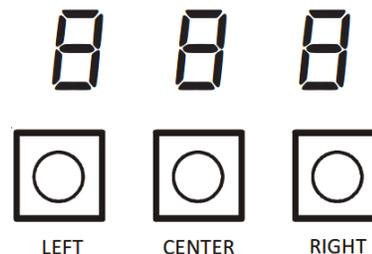
The air handler includes three on-board push buttons allowing users to navigate indoor and outdoor system menus. The Right and Left buttons allow the user to scroll through the main menus and to then scroll through available options within specific menus. The Center button is used to enter into a main menu and to then permanently select options within those menus.
