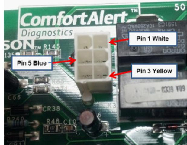
4. If voltage is present at these pins plug harness into plug on PC board and check voltages at motor to test for broken wires.
