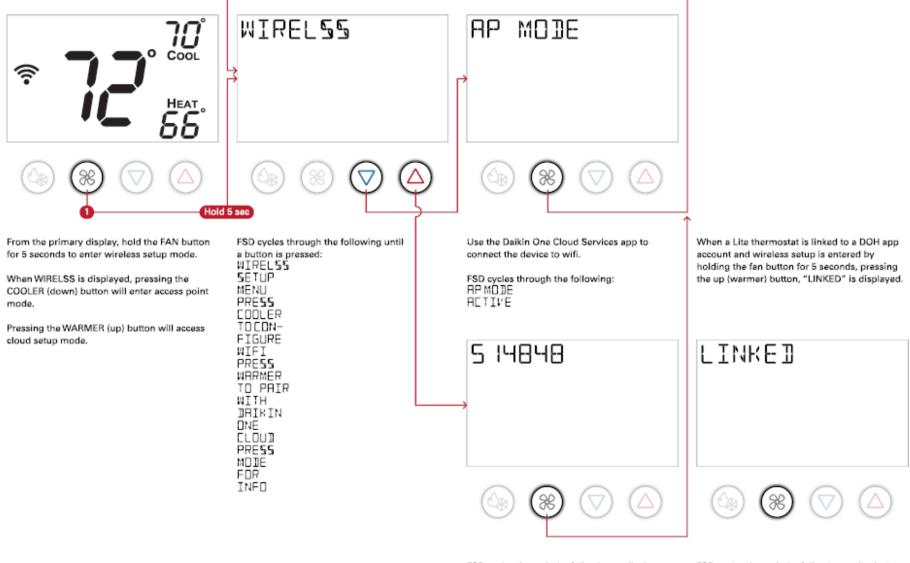
FSD cycles through the following until a button is pressed:
