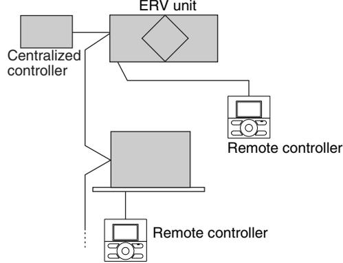
• Interlocking system with VRV or SkyAir system
