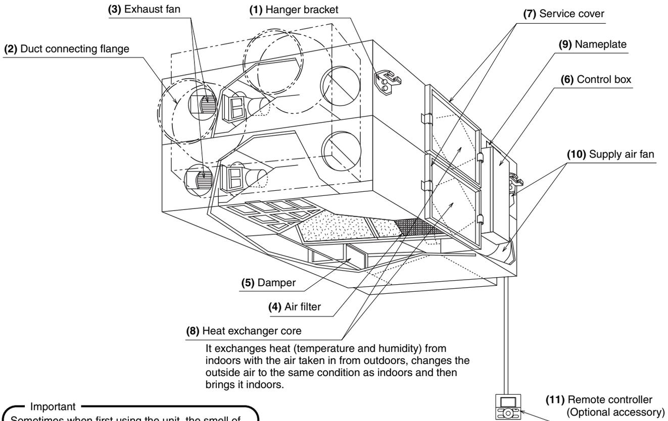
It exchanges heat (temperature and humidity) from indoors with the air taken in from outdoors, changes the outside air to the same condition as indoors and then brings it indoors.
