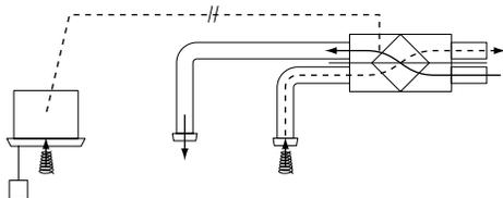
The ERV unit cannot be operated independently when the air conditioner is connected to the ERV unit via a duct. When using the ERV unit, set the fan speed of air conditioner to “Low”.
