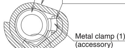
Wrap the sealing material (Large) (6) so that the metal clamp (1) end side may be doubled.
