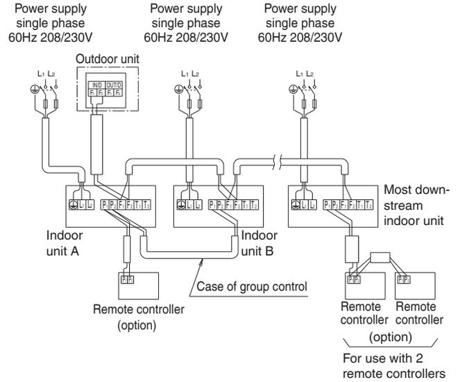
Note) There is not need to set the indoor unit address when using group control.
