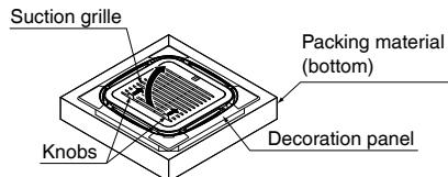
(2) Open the suction grille to an angle of approximately 45° and remove the suction grille from the panel.
