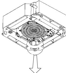
(1) Remove the bypass hole closing cap.
