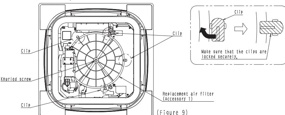
(3) Return the brush unit to its original position by reversing steps <4>-(1) through -(5) above and tighten the knurled screw.
