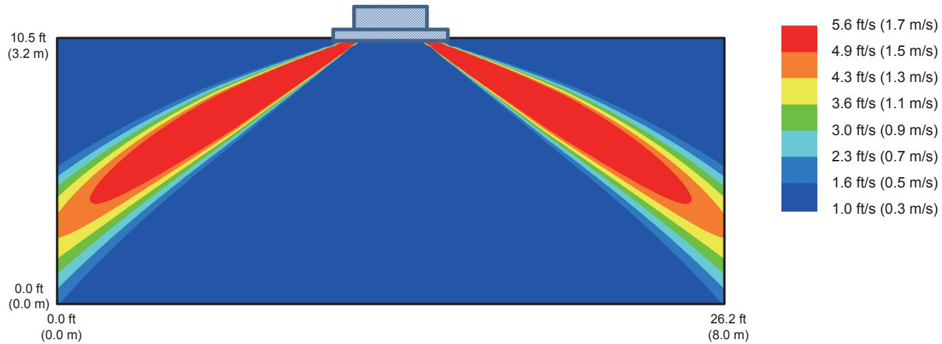
**Air temperature distribution of F XFQ36TVJU (Cooling operation)**
