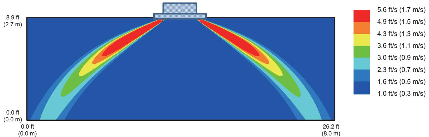
**Air temperature distribution of F XFQ15TVJU (Cooling operation)**
