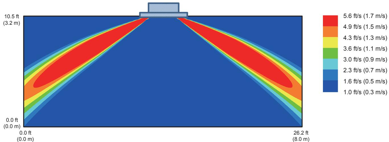
**Air temperature distribution of F XFQ48TVJU (Cooling operation)**
