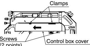
Loosen the screws (in 2 points) and slide the control box cover in the direction of the arrow to unhook the cover from the clamps.
