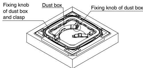
(1) Turn the 2 fixing knobs of the dust box.
