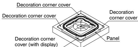
(1) Raise and remove the decoration corner cover (with the display) in the direction of the arrow.
