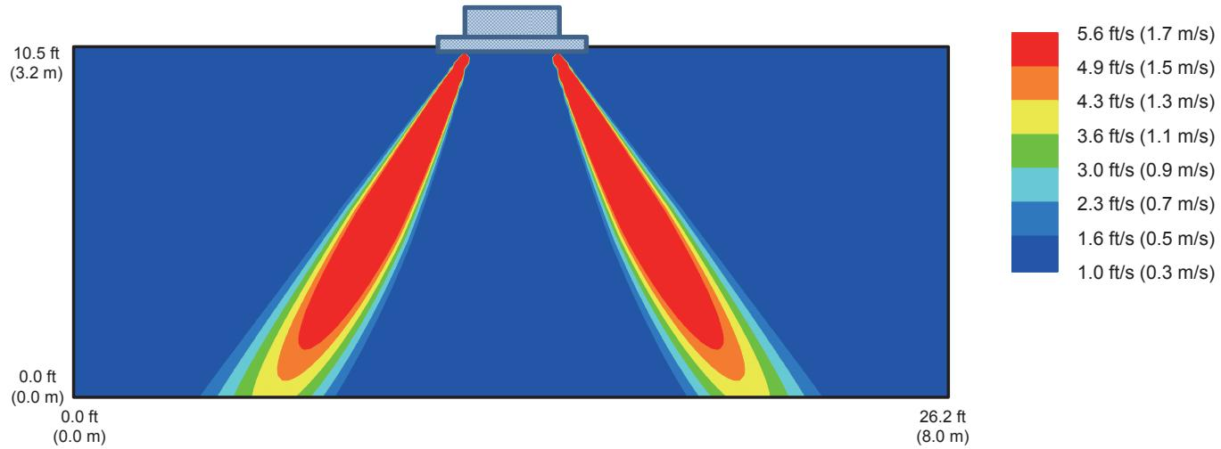
**Air temperature distribution of F XFQ36TVJU (Heating operation)**
