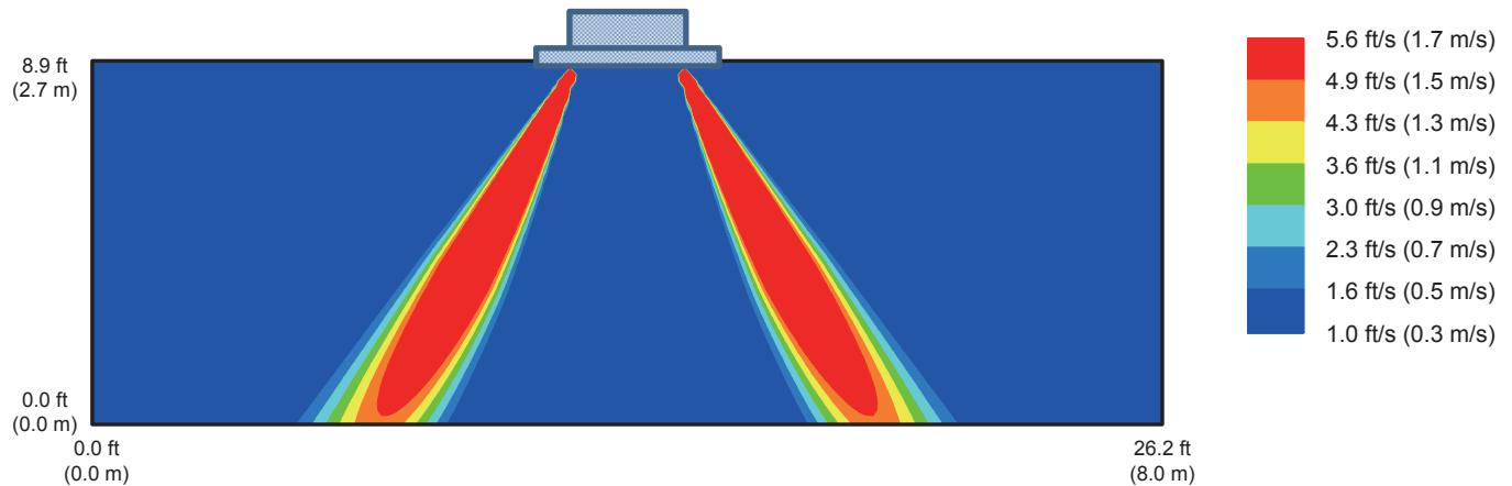
**Air temperature distribution of F XFQ30TVJU (Heating operation)****Air flow direction : Down**
