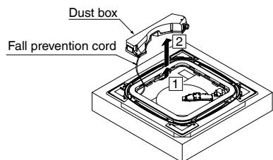
(3) Remove the fall prevention cord for the dust box from the clasp bracket of the panel.
