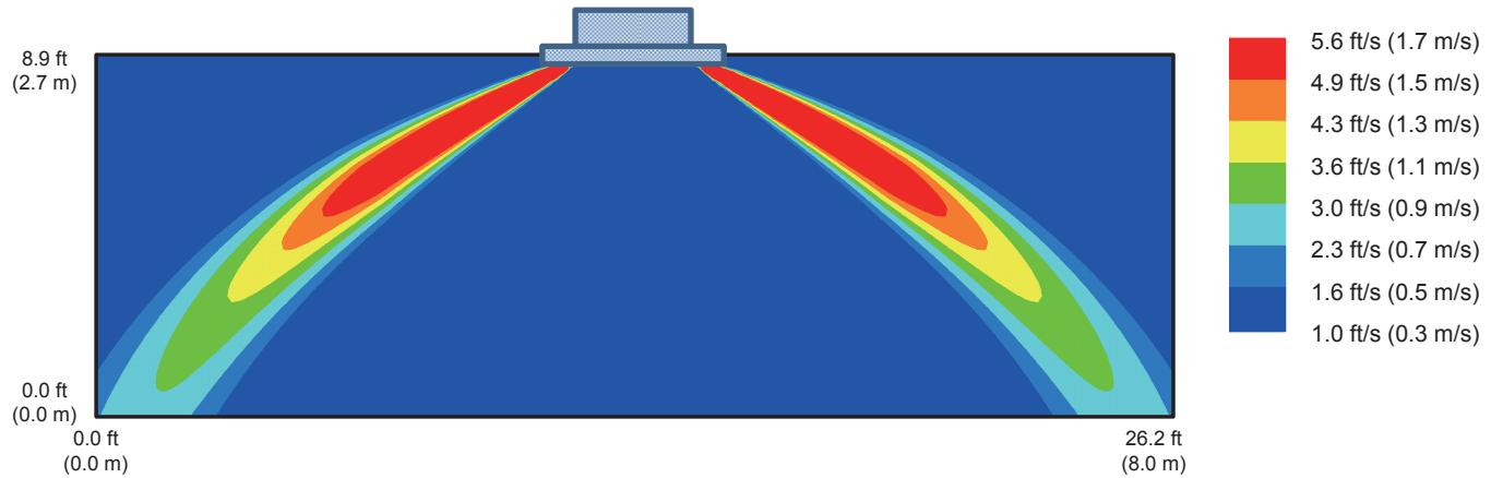
**Air temperature distribution of F XFQ24TVJU (Cooling operation)**
