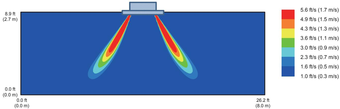
**Air temperature distribution of F XFQ09TVJU (Heating operation)**
