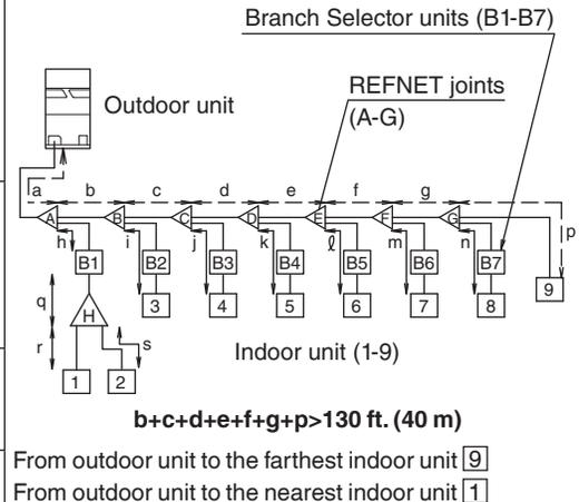
In the case of a multi Branch Selector unit, if a junction pipe kit (separately sold) is used for combining 2 lines, the actual piping length between the multi Branch Selector unit and the indoor units should be  $\leq 65$  ft. (20 m).
