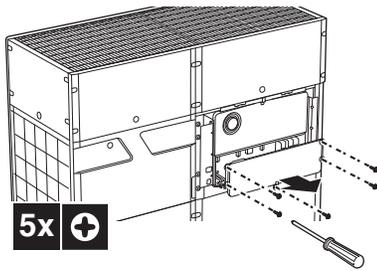
For service purposes, the push buttons on the main printed circuit board need to be accessed. To access these push buttons, the control box cover does not need to be opened. See 13. Making field settings on page 26.
