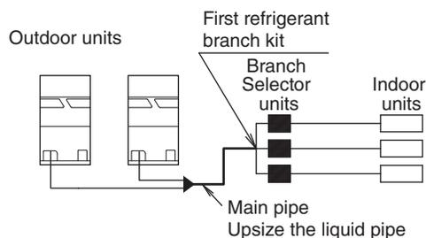
(\*7) Vertical height difference between outdoor units and indoor units can be extended to  $\leq 361$  ft. (110 m) with liquid piping of main pipe upsize (see the figure and table above). See [2-49]=Height difference setting on page 36.
