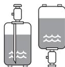
If a siphon tube is not equipped, change the liquid refrigerant with the cylinder in upside-down position.
