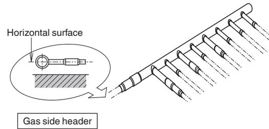
Mount the REFNET header so that the branch pipes are on the underside and branch horizontally.
