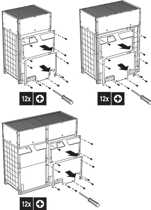
Once the front panel open, the control box can be accessed by removing the control box cover as follows.
