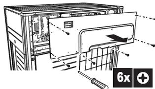
For service purposes, the push buttons on the main printed circuit board need to be accessed. To access these push buttons, the control box cover does not need to be opened. See 13. Making field settings on page 24.
