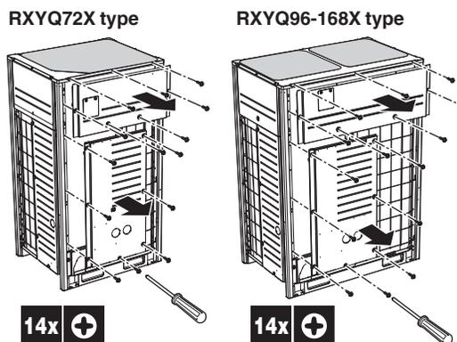
Once the front panel open, the electrical component box can be accessed by removing the control box cover as follows.
